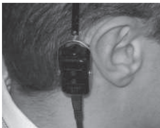
Figure: placement of bone vibrator on mastoid during bone conduction testing
