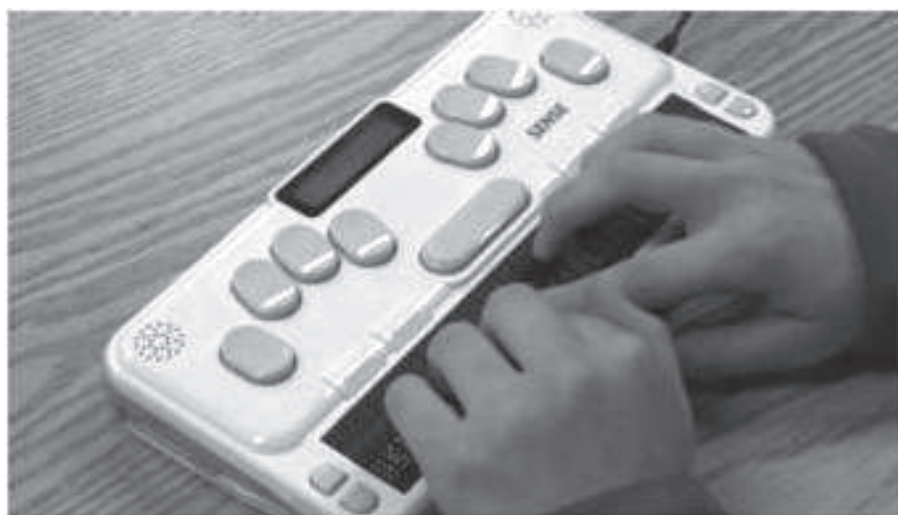
Figure 15: Braille Notetaker (Source: Florida School for the Deaf and the Blind in St. Augustine, Florida-Video Library)
