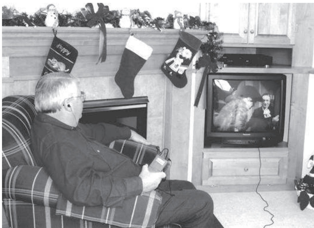
Figure 7: A “personal communicator” amplifier to enhance communication in the absence of custom hearing amplification. The device may be plugged directly into the television set or other audio-output jacks to provide direct sound to the user’s ear thereby improving the signal-to-noise ratio. With a plug-in microphone, such devices can also be invaluable in helping to maintain more private conversations between healthcare providers and their patients in compliance with privacy legislation. (Courtesy of Williams Sound Corporation)
